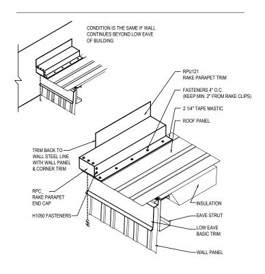
NOTE: ALL POP RIVETS AND FASTENERS ARE TO BE SET "IN" THE MASTIC OR CAULK
